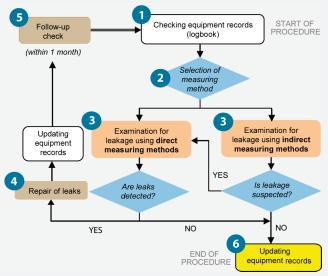
Steps 1 to 3 must be carried out always. If no leaks are suspected (indirect measuring methods) or detected (direct measuring methods), the procedure is completed by updating the equipment records (logbook) (step 6).
